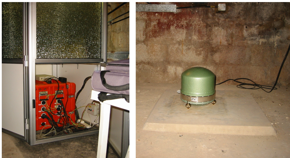
Figure 2: WDD seismic station. Left: The Quanterra Q680 data acquisition system. Right: The Streckeisen triaxial seismometer placed on a concrete platform.
